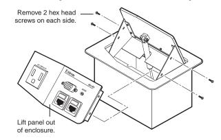
Figure 3-6 — Front panel removal (HSA 200 models)
